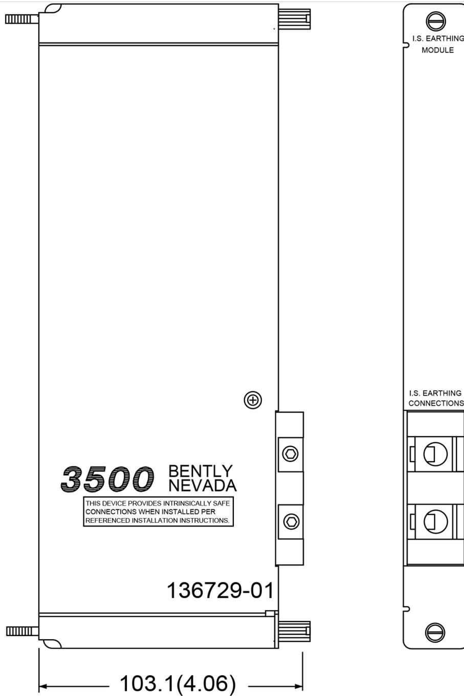
**Figure 2: Rear Views of the 3500/04-01 Internal Barrier Earthing Module**
