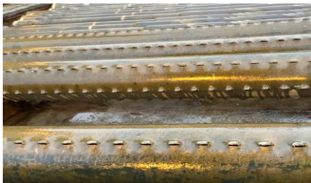
Slotted 13-3/8 in. casing
