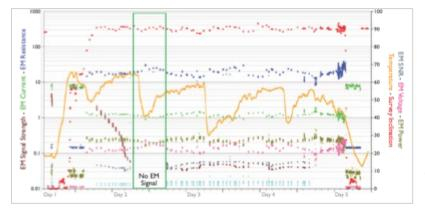
NaviTrak UT allowed the directional team to rely on mud pulse when the EM signal was lost, eliminating the need to POOH for MWD or spend time downlinking to change telemetry.
