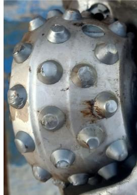
1,418 ft drilled with abrasion resistant Clear Lake carbide
