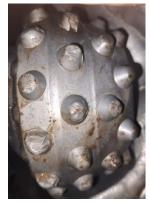
705 ft drilled with general purpose Clear Lake carbide
