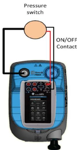
**Figure 4-1: Switch testing setup**
