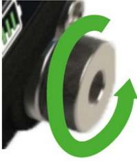
The pressure release knob is on the bottom right of the instrument. To release pressure, slowly turn the valve knob counterclockwise one full rotation. Make sure the system is sealed before pressure generation: fully turn the pressure release knob in the clockwise direction to close.
