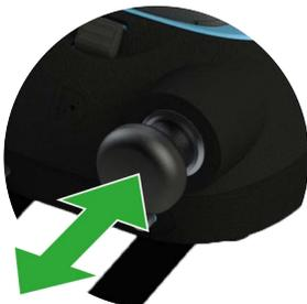
When you have set the operation mode to pressure or vacuum, seal the system (Section 3.5). Move the pump handle forwards and backwards to pressurize the instrument or make a vacuum.
