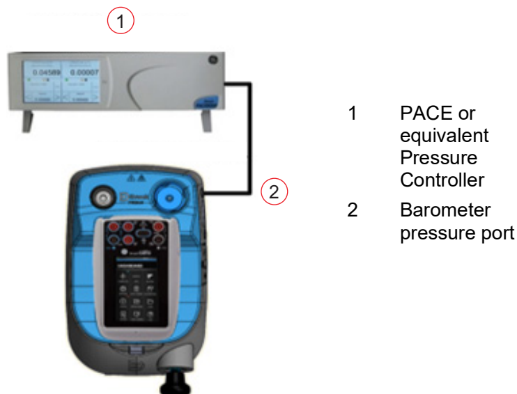
Figure 4-6: Barometer Calibration Setup
