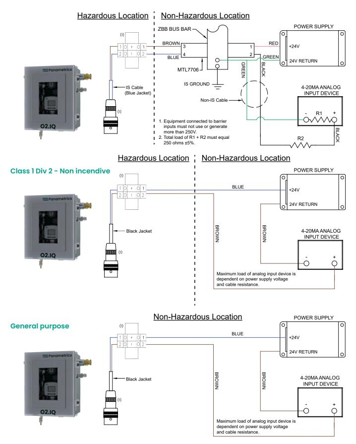
Note: Wiring to integrated terminal strip to be completed at installation site. oxy.IQ connection cable ships separately.
