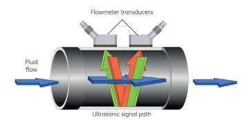
With transit time flow measurement, two transducers serve as both ultrasonic signal generators and receivers. When mounted on a pipe, they are in acoustic communication with each other, meaning the second transducer can receive ultrasonic signals transmitted by the first transducer and vice versa.
