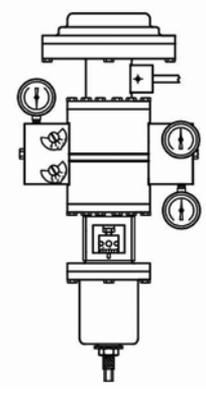
**Figure 6.4 - Model HPP-4 Direct-Acting Positioner (Split Range)**
