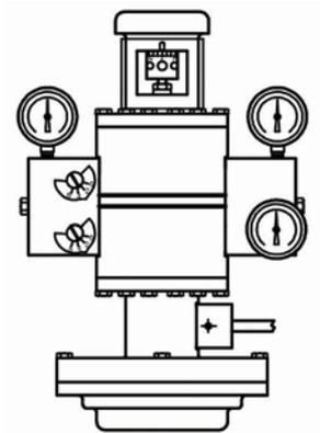
**Figure 6.1 - Model HPP-4 Reverse-Acting Positioner (Standard Range)**
