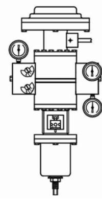
**Figure 6.4 - Model HPP-4 Direct-Acting Positioner (Split Range)**
