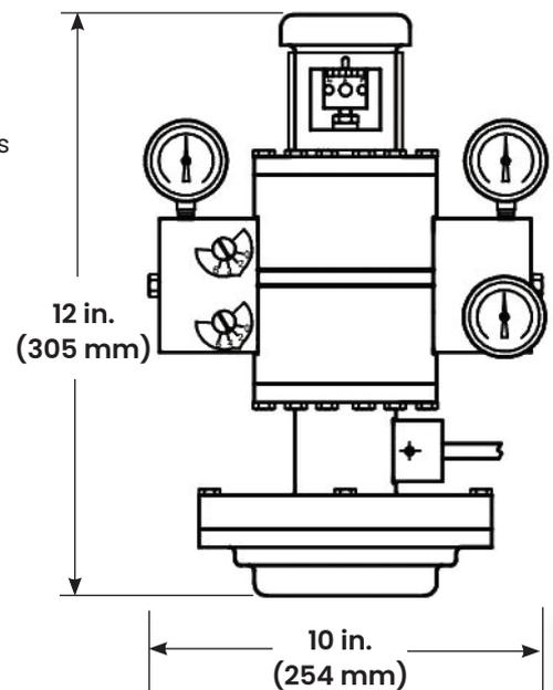
**Figure 5 – Overall dimensions of HPP-4 positioner (standard range)**
