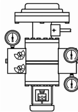
**Figure 6.3 - Model HPP-4 Direct-Acting Positioner (Standard Range)**
