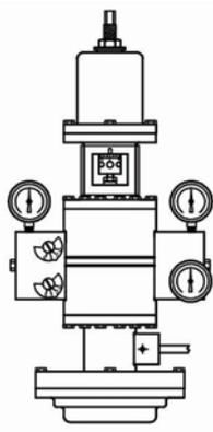
**Figure 6.2 - Model HPP-4 Reverse-Acting Positioner (Split Range)**
