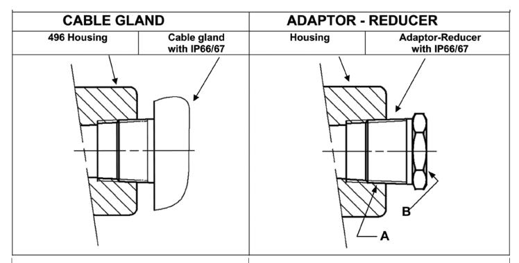
TYPE: Male Taper (conical) threaded joint: 3/4" NPT
