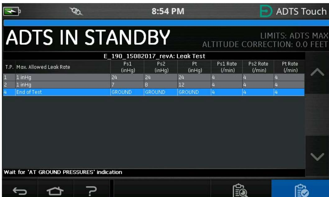
The screenshot shows the ADTS Touch interface in standby mode. The title is "ADTS IN STANDBY" with "LIMITS: ADTS MAX" and "ALTITUDE CORRECTION: 0.0 FEET" on the right. The test sequence is titled "E\_190\_15082017\_revA: Leak Test". The table below shows the test points with row 4 highlighted in blue. A blue arrow on the right indicates scrolling down.
