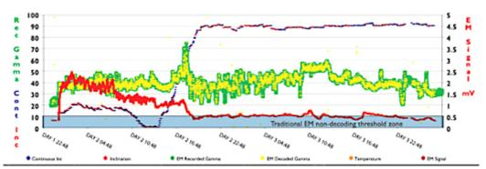
NaviTrak<sup>™</sup> UT provided high-quality gamma and increased average ROP by 29 ft/hr, a 15% increase compared to conventional mud pulse.
