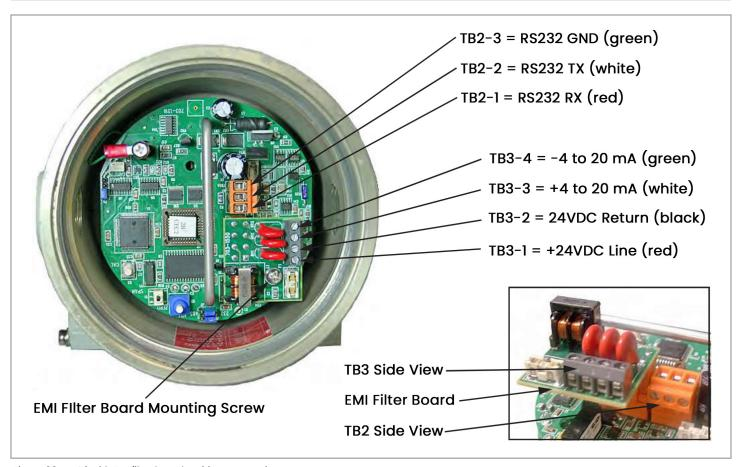
Figure 88: XMO2 with EMI filter board - wiring connections
