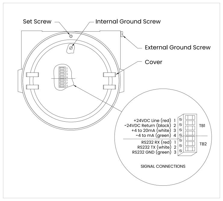
Figure 7: TB1 and TB2 terminal block connections
