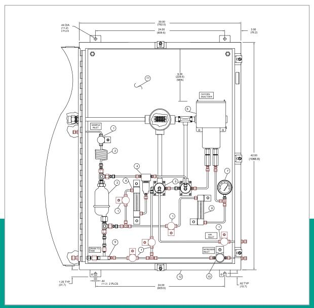
Figure 59: Blanketing gas sample system
