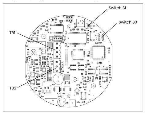
Figure 11: PCB calibration switches
