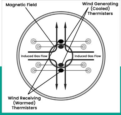
Figure 2: Arrangement of the thermistor pairs
