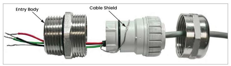
Figure 89: Proper cable gland assembly (Panametrics p/n 419-215)
