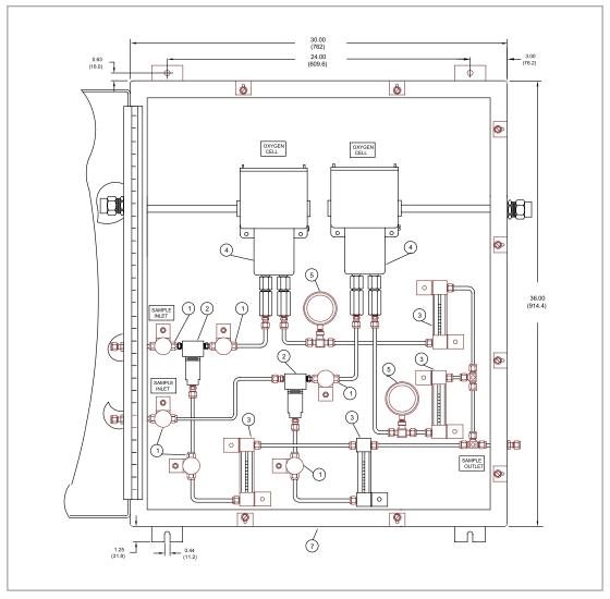
Figure 60: Formaldehyde feed gas sample system
