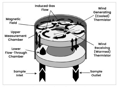
Figure 1: Measuring cell flow schematic
