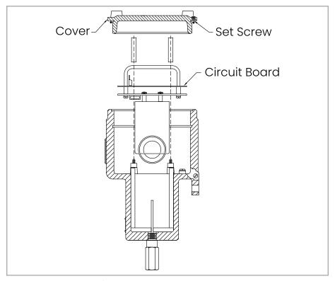
Figure 10: XMO2 Cover, set screw, and PCB
