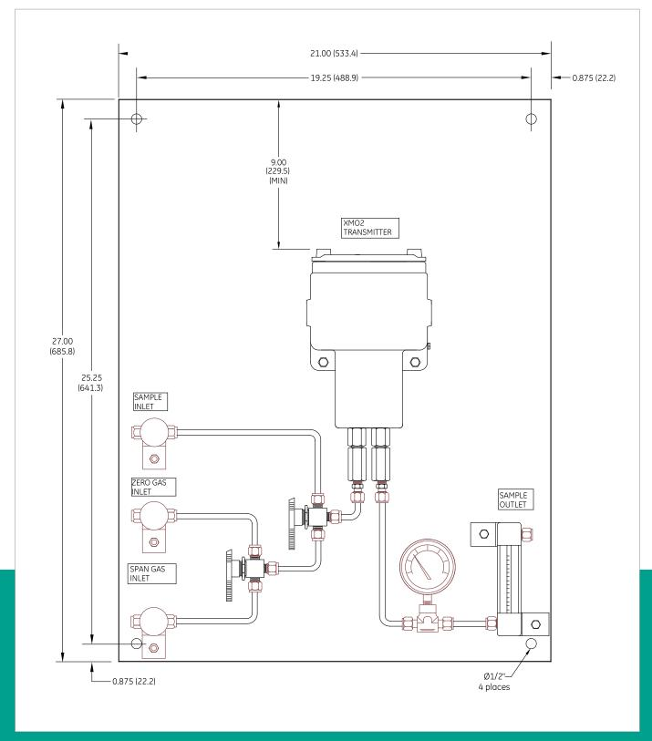
Figure 5: Basic XMO2 sample system (ref. dwg #732-164)
