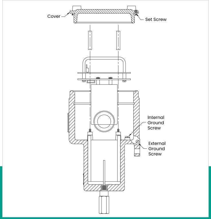
Figure 6: XMO2 Ground screw locations
