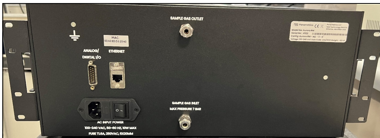
Figure 6: Rear panel showing Power, Certification, and Sample Inlet Labels.
