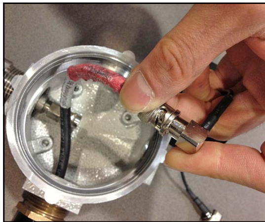
Figure 11: Connecting BNC Plug to Cable
