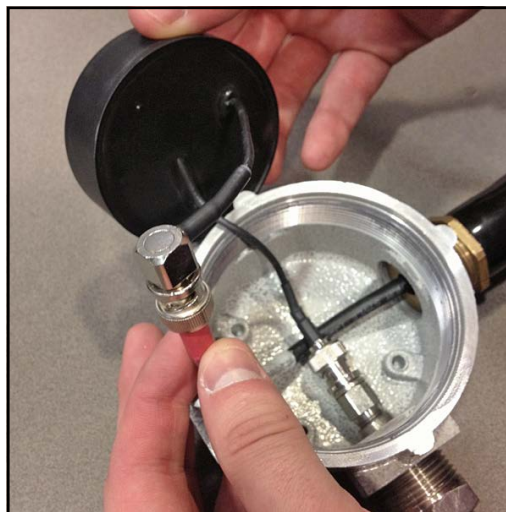
Figure 12: Female Plug to Male BNC Head
