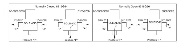
Figure 15: Schematic Wiring Diagram Electromatic Valve 220 VDC and 250 VDC
