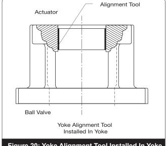
Figure 20: Yoke Alignment Tool Installed In Yoke
