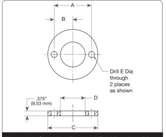
Figure 26: Stem Nut Removal Tool Retainer Plate
