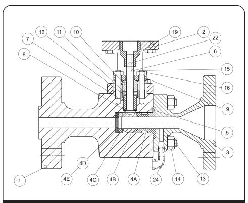
Figure 2: 3500 Valve Typical Flange Inlet.
