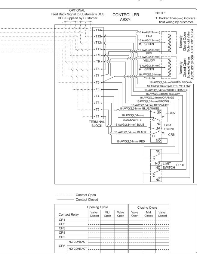
Figure 14 (Cont.): Schematic Wiring Diagram Electromatic Valve 120VAC, 240VAC, 24VDC, and 125VDC
