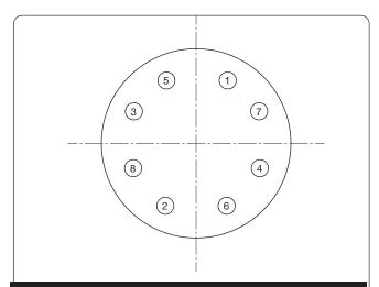
Figure 18: Discharge Collar Torquing Pattern
