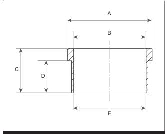
Figure 27: Yoke Alignment Tool Machine Drawing
