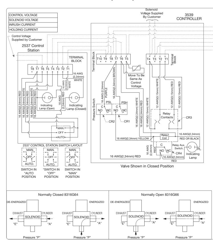
Figure 14: Schematic Wiring Diagram Electromatic Valve 120VAC, 240VAC, 24VDC, and 125VDC
