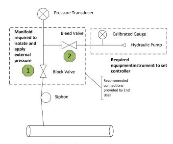
Pressure sensing connection should be located at least 8 to 10 pipe diameters upstream from the EBV
