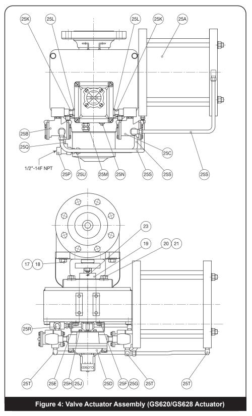
Note: The drive bushing that connects the LEDEEN GS620 and 628 actuators with the stem of the ball valve may float up inside the actuator during re-assembly. A temporary application (during disassembly), of duct-tape or a 4" hose clamp will hold it in position with about 3/4 of an inch of bushing showing below the actuator. Following re-assembly remove any ducttape or hose clamp from the drive bushing and ensure that the drive bushing set screw is tight.
