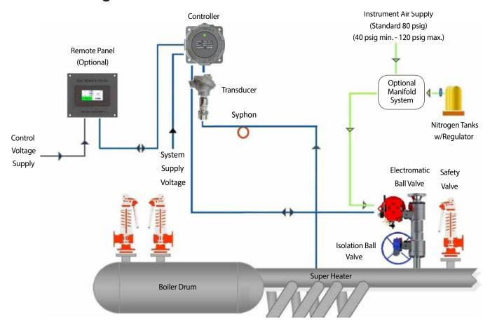
Figure 1: Typical Electromatic Ball Valve System
