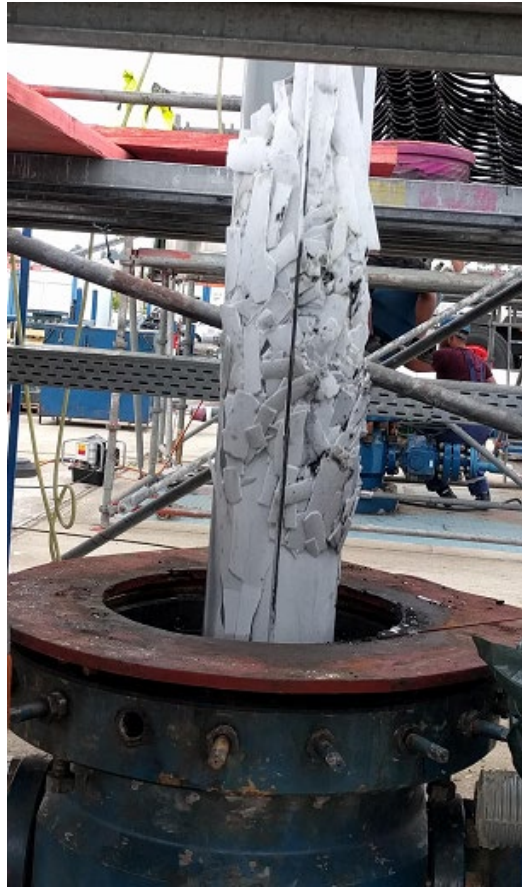
Figure 18-1: An ESP being pulled from a scale intensive well in Southern Germany
