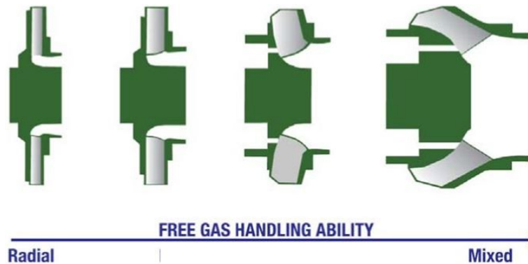
Figure 5-1: Free gas handling ability by stage type
