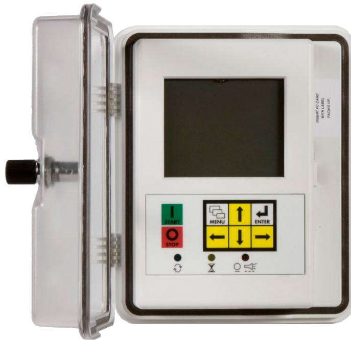
Figure 11-3: Graphical control system (GCS) display
