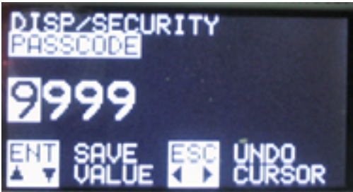
Figure 42: Security check window
