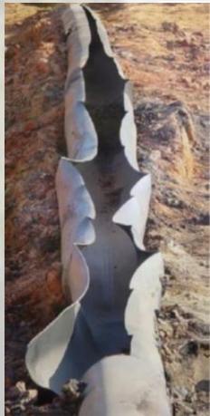
Figure 3-2: Visualization of fracture propagation vs arrest in steel pipelines
