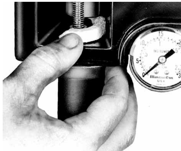
Figure 18 - Adding a packing ring
