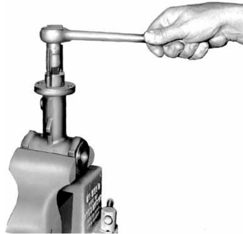
Figure 19 - Tightening the seat-ring retainer (4)
