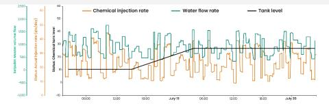
The InjectRT service instantaneously aligns chemical injection rates with ESP-derived virtual flow rates
