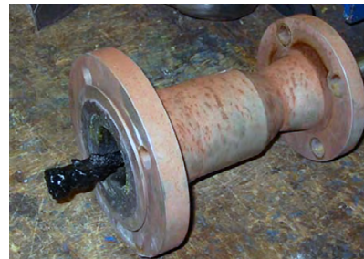
Figure 4. Upstream transducer removed for inspection
