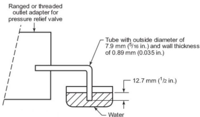
Figure 2. Apparatus to test seat tightness with air.
