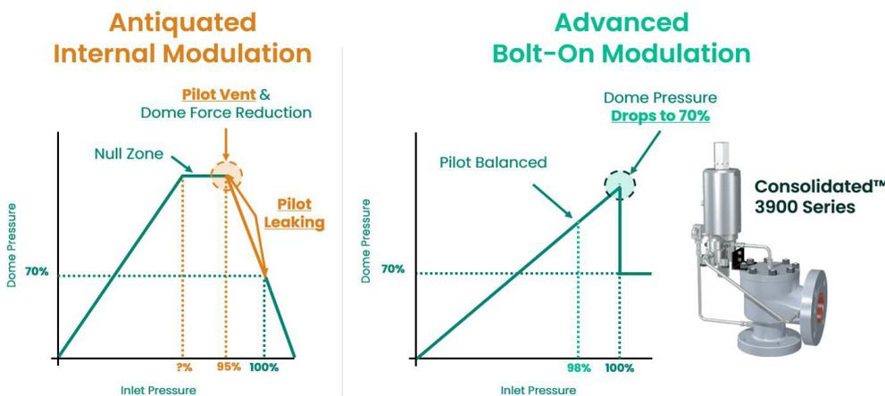
**Figure 3. Antiquated internal modulation vs advanced modulation technology.**
