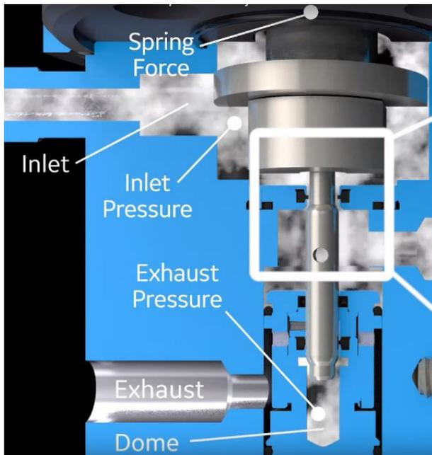
**Figure 4.** Internal modulation diagram.
