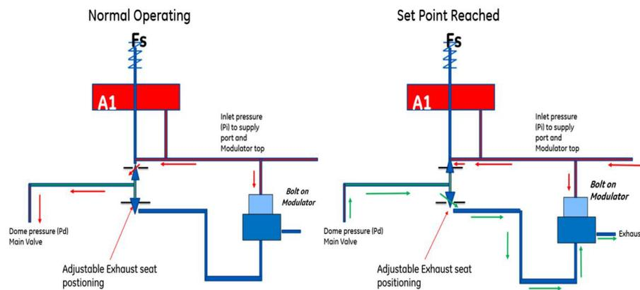
**Figure 5.** Bolt-on modulation diagram.
