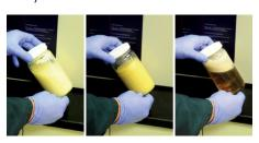
The GelBlock system is engineered and pumped as a viscous slurry. Shortly after exposure to downhole temperatures, it hardens into a solid that can be used for temporary isolation of a zone. Then, after pumping a breaker, the hardened material becomes a low-viscosity liquid which is easily circulated out with the production flow.
