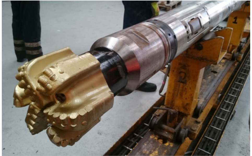
The AutoTrak eXact system's bottomhole assembly (BHA) featured a custom Talon Force bit with EZCurve technology and StaySharp cutters to provide superior steering performance in the chalk formation.
