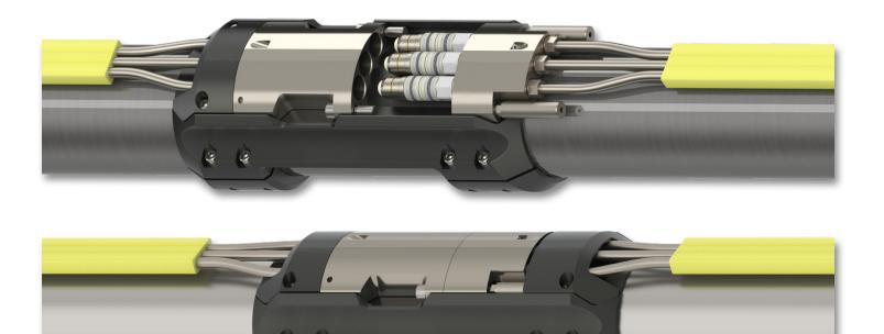
The UpCable dry-mate field-connect socket and field-connect plug eliminate splicing to reduce risk and installation time from hours to minutes, increase reliability and extend service life. Key features include pressure test ports, an oil filled pressure compensated connector, metal to metal sealing, a non-elastomeric backup seal stack, and metal bellows pressure compensator/intensifier.
