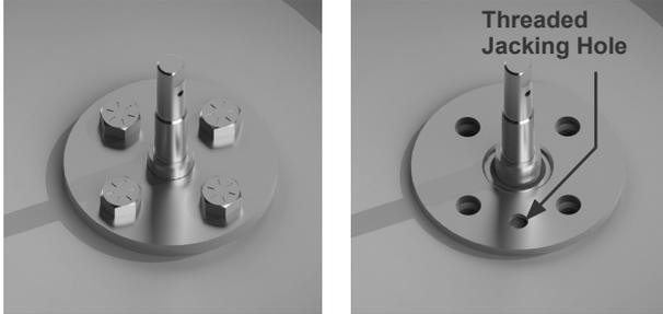
12. Thread two of the Seal Pack cap screws into the extra holes and tighten to lift the Seal Pack out of the Lower Actuator Housing.
