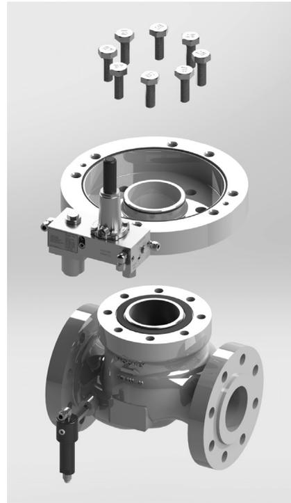
26. Remove the Upper Crush Gasket and lift the Cage from the Body. Clean and inspect the Cage for any sign of abrasive wear or damage.
