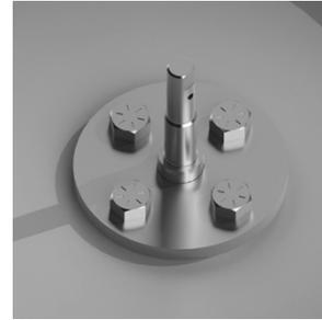
36. Install Lower Diaphragm Support plate, Diaphragm, and Upper Support plate.
