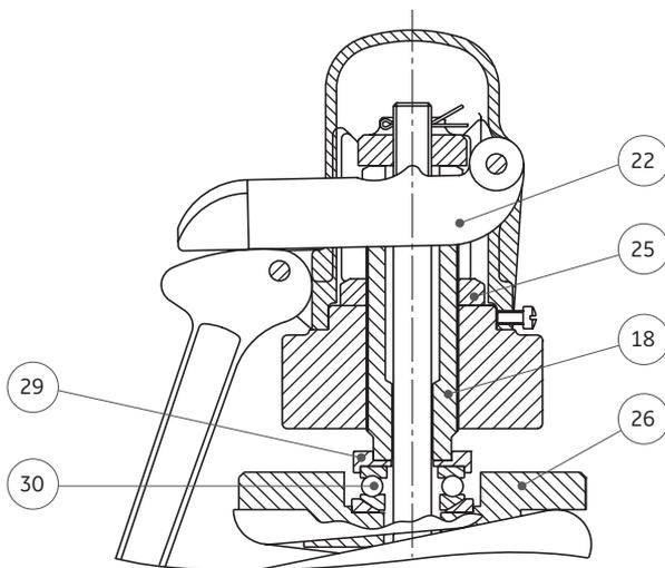
Figure 4: Thrust Bearing
