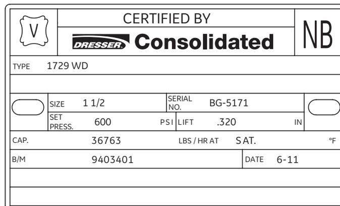
Figure 38: Valve Nameplate
