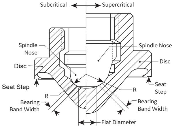
**Figure 24: Disc - Spindle Assembly**
