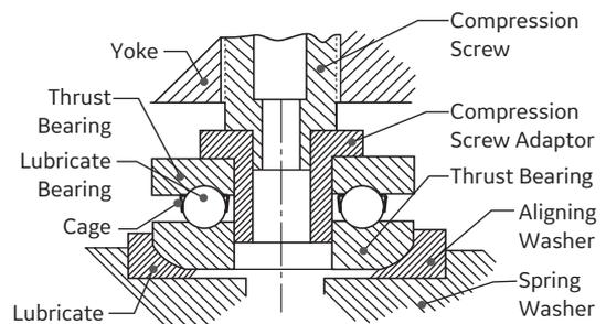
Figure 27: Thrust Bearing Assembly
