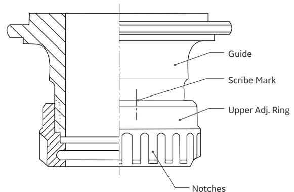
**Figure 15: Upper Adjusting Ring and Guide Assembly**
