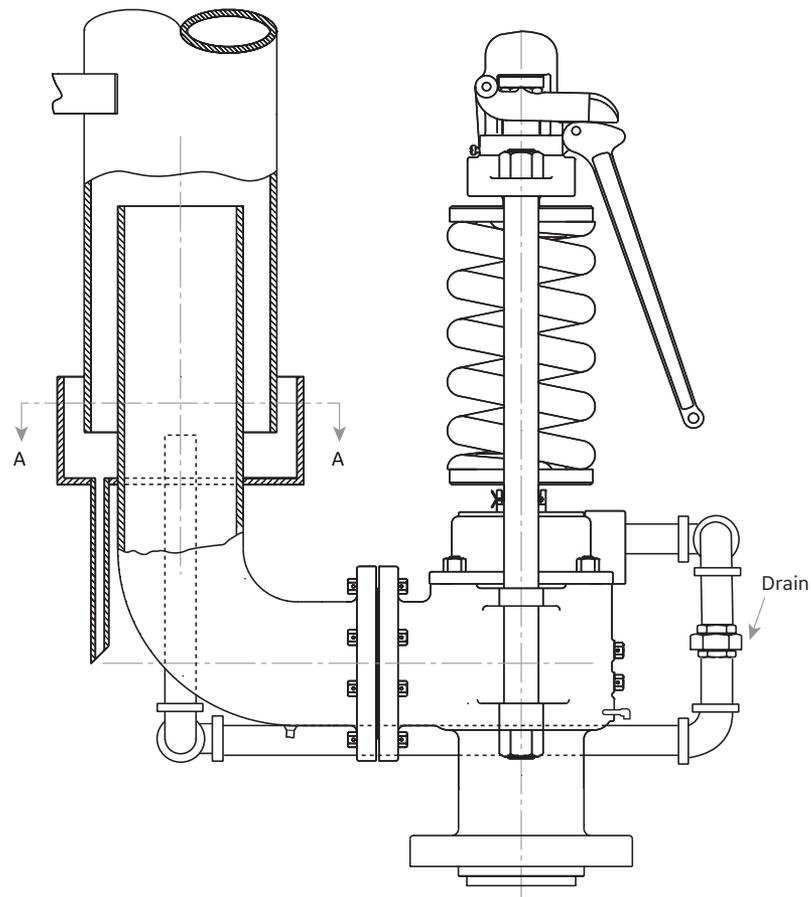
Figure 10: Recommended Installation
