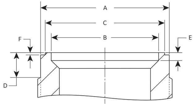
Figure 20: Seat Bushing Dimensions
