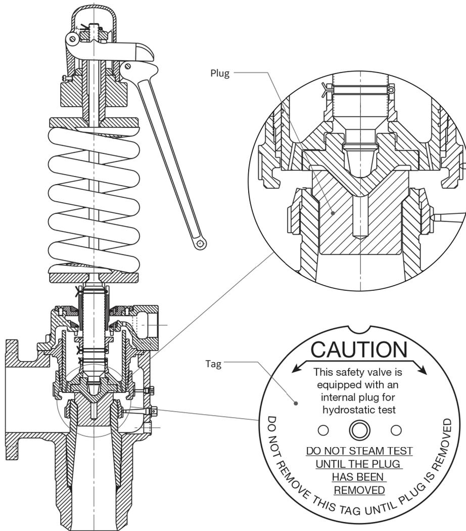
**Figure 36: Hydrostatic Test Plug**
