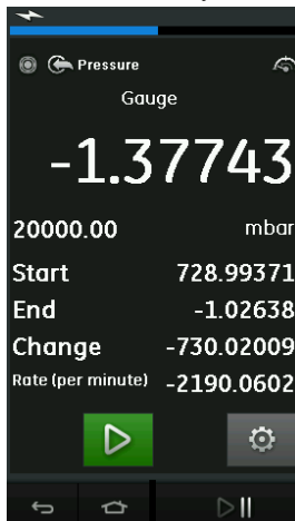
Figure 2-26: Leak Test Example
