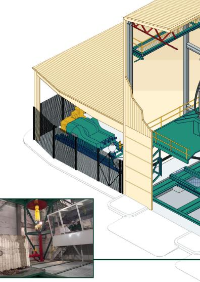
Our full-scale atmospheric pressure test rig facilitates wear and dynamic analysis of all types of drill bits.
