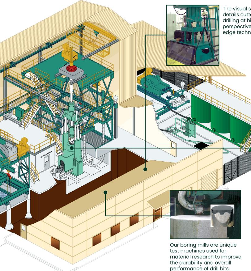
The visual single-point cutter machine details cutter/rock interaction during drilling at high pressures. Its unique perspective brings fresh ideas to cuttingedge technology and drilling efficiency.
