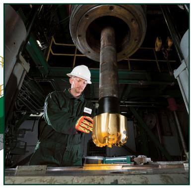
Our full-scale, high-pressure bottomhole drilling simulator brings the field into the laboratory, significantly reducing new bit development from months to days.
