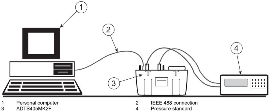
**Figure 5-1: Automatic Calibration Arrangement**
