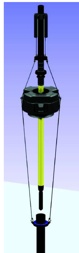
Figure 1: T-CAT tool showing how the slings are attached to the cylinders and to the single joint elevator, as well as the position of the FAC tool stinger before it is pulled into the casing.
