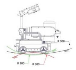
For in-vessel inspection a minimum vessel radius of 300 mm (11.8") is mandatory. This allows for axial driving. Full maneuverability, incl. spot turn is possible at a radius of 900 mm (35.4").
