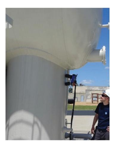
In this framework, the BIKE inspection robot has been developed. The BIKE platform is a magnetic wheeled robot capable of inspecting power plant facilities and multiple applications in the oil & gas industry, such as vessel or pipe inspection. The innovative locomotion concept allows climbing obstacles such as stairs and 90 degree corners (convex & concave).
