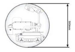
Minimum size of entryway for safe deployment and retrieval of the inspection system is 500 mm (20").
