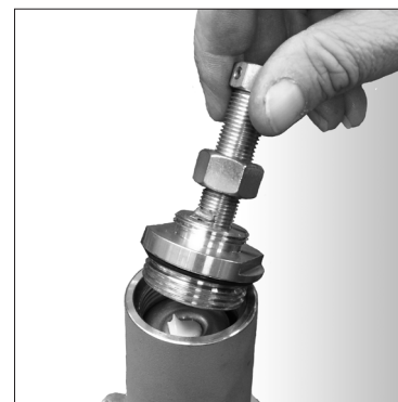
Figure 16 Installing the closing cap assembly for Pilot with the Red, Plated, Blue, and Purple Springs
