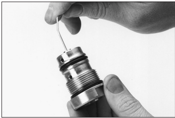
Figure 11 The orifice can be pushed out of the Body Insert (Cartridge) using a paper clip
