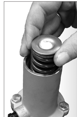
Figure 15 Installing the Spring with lubricated Spring Follower
