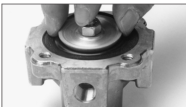
Figure 13 Placing Diaphragm Assembly on Pilot Body
