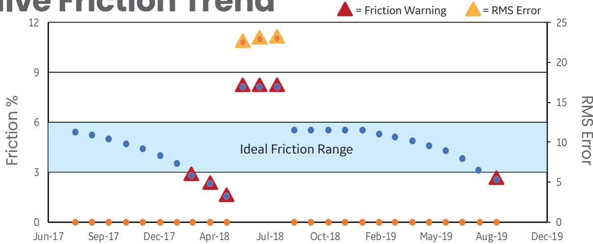
Packing friction reduction observed over time. May '18 Technician over-tightens packing and increases RMS error. Aug. '18 packing loosened to improve RMS. Aug. '19 Alert for low packing friction - potential for fugitive emissions.
