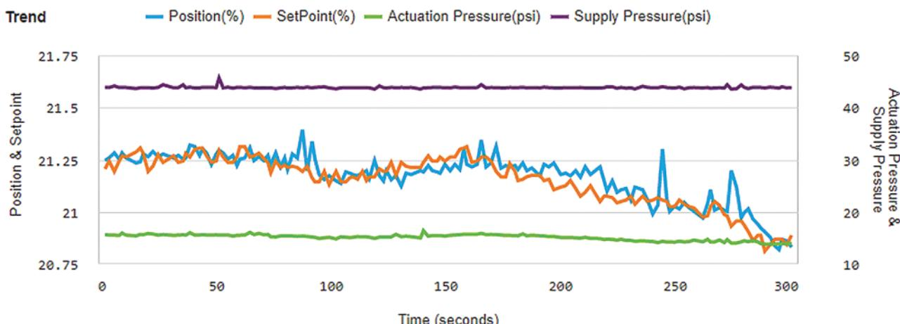
Valve is responsive and tracking closely to set point for precision control. No outliers identified.
