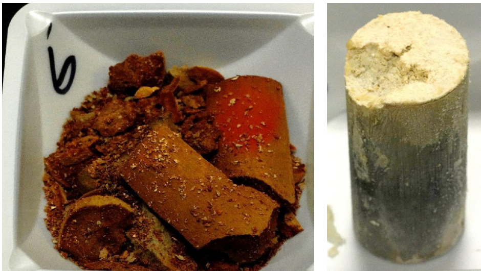
Figure 1: Comparison of TerraSet (Right at 4 weeks) vs. conventional OPC design (Left at 2 weeks) after curing in 4M in acetic acid as an analogue to H_2O/CO_2 generated carbonic acid. 190°F and ambient pressure.
