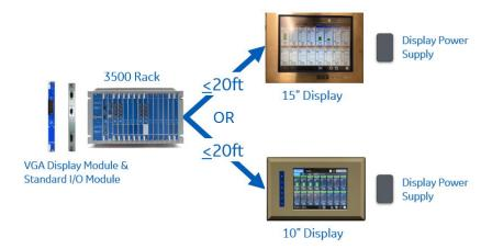
Figure 3: Single Rack with 10" or 15" Remote Display
