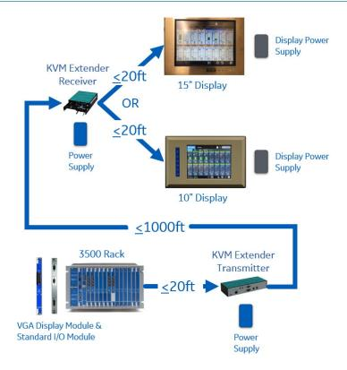
Figure 4: Single Rack with KVM Extender
