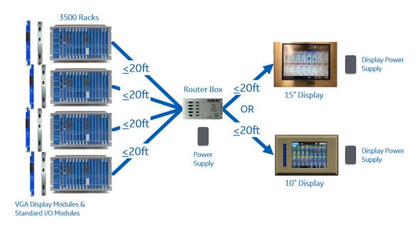
Figure 5: Multiple Racks with Router Box
