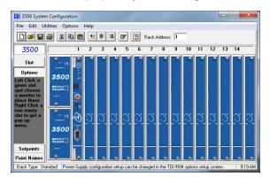
3500 System Configuration Software can be run on a laptop computer, which is connected locally to the USB port on the face of the TDI, or on a remote computer, which is connected to the TDI via the plant network. Configuration settings include the following:
