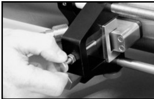
Figure 1-10: Installing the First Transducer
