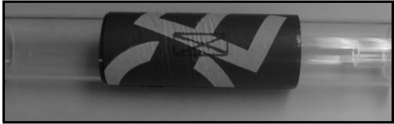
Figure 1-23: DMP-1 Material with Transducer Footprint Traced
