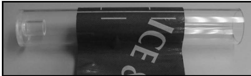
Figure 1-22: DMP-1 Damping Material Wrapped Around Pipe
