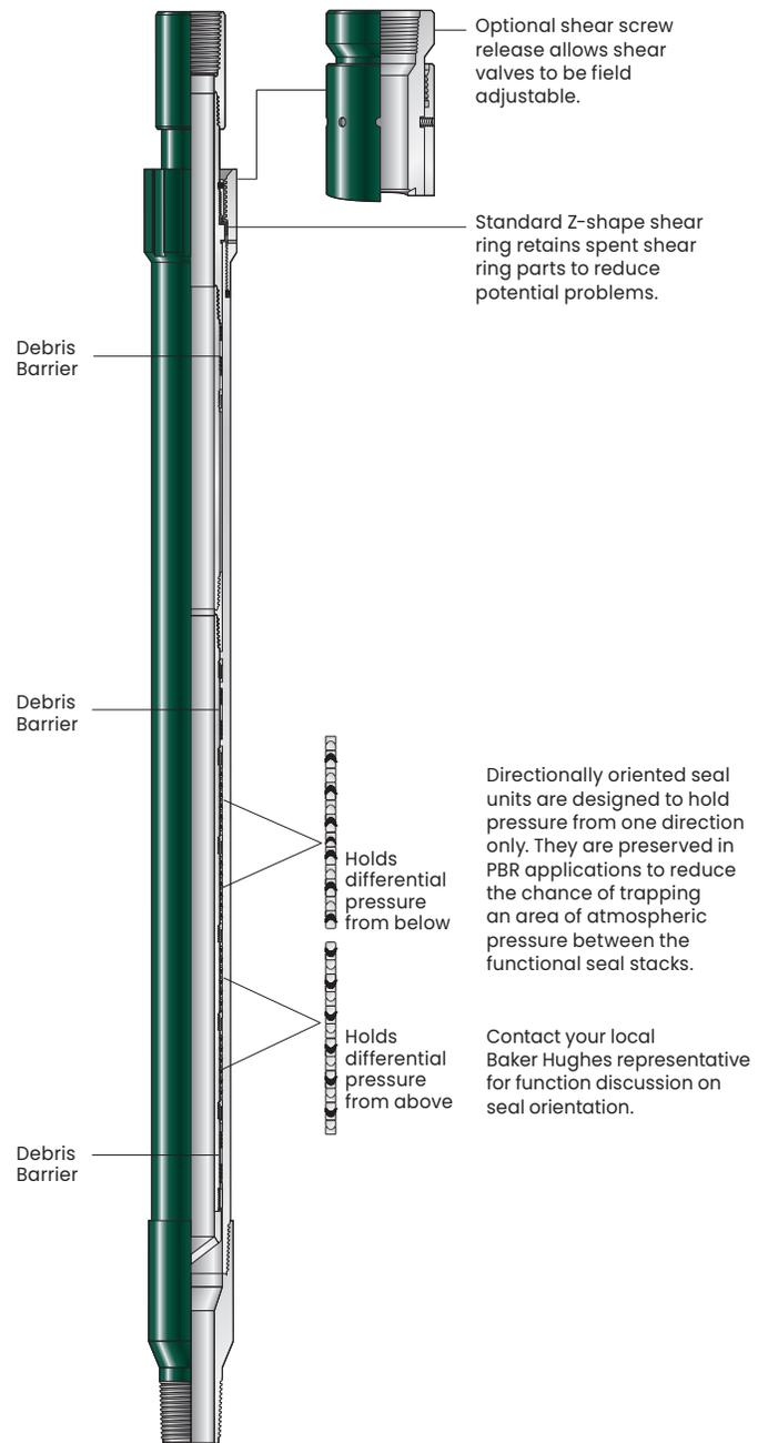
*Non-sealing debris barriers serve two important functions: they keep well solids or trash from setting in the annular area between the honed bore and seal assembly which may impede the movement of the seal assembly. They also clean the sealing area before functional working seals contact the sealbore.*
