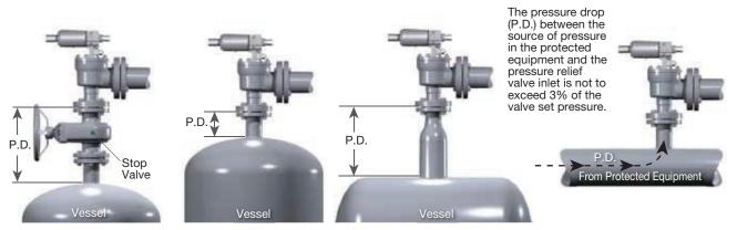
Figure 9: Pressure Drop on the Inlet Piping
