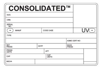
Figure 46: Nameplates for Main Valve
