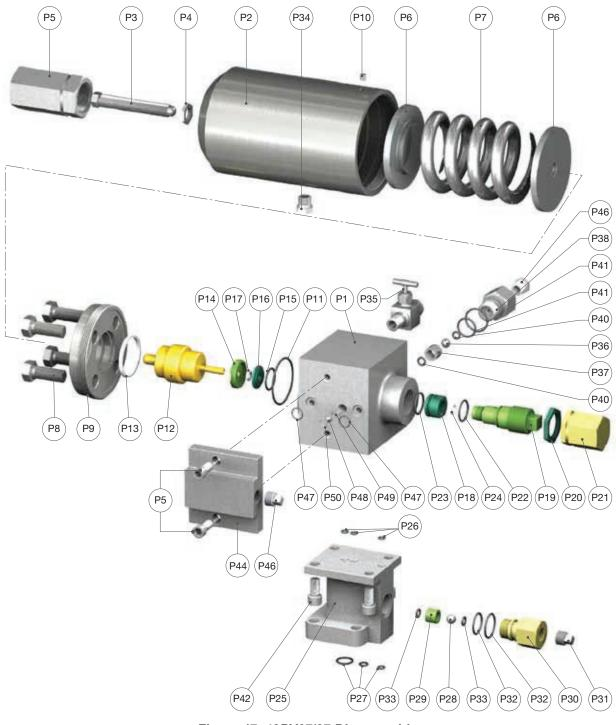
Figure 17: 49PV07/37 Disassembly
