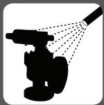
Decontaminate or clean if necessary before pretesting or disassembly. Safety and environmental precautions must be taken for the decontamination or cleaning method used.
