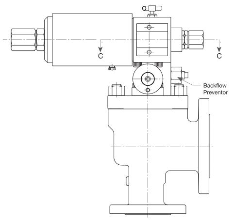
Figure 2: 4900 Series POSRV Assembly with 49PV07/37 Pilot
