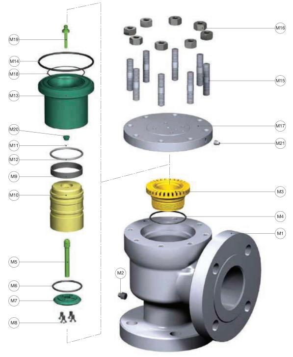
Figure 12: POSRV Assembly with MV22/72 Pilot
