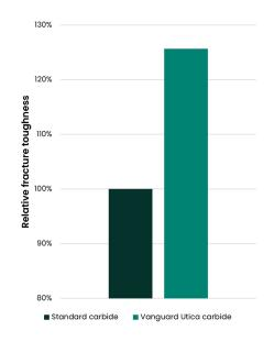
The Vanguard Utica's advanced carbide inserts demonstrate superior fracture toughness for longer run life compared to standard carbide grades.
