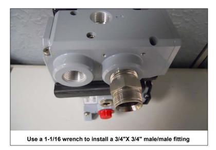
Figure 68 - Step 1 Install a 3/4" x 3/4" Fitting
