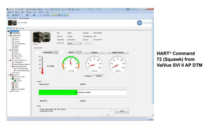
Figure 38 - HART<sup>®</sup> Command 72 Squawk Function
