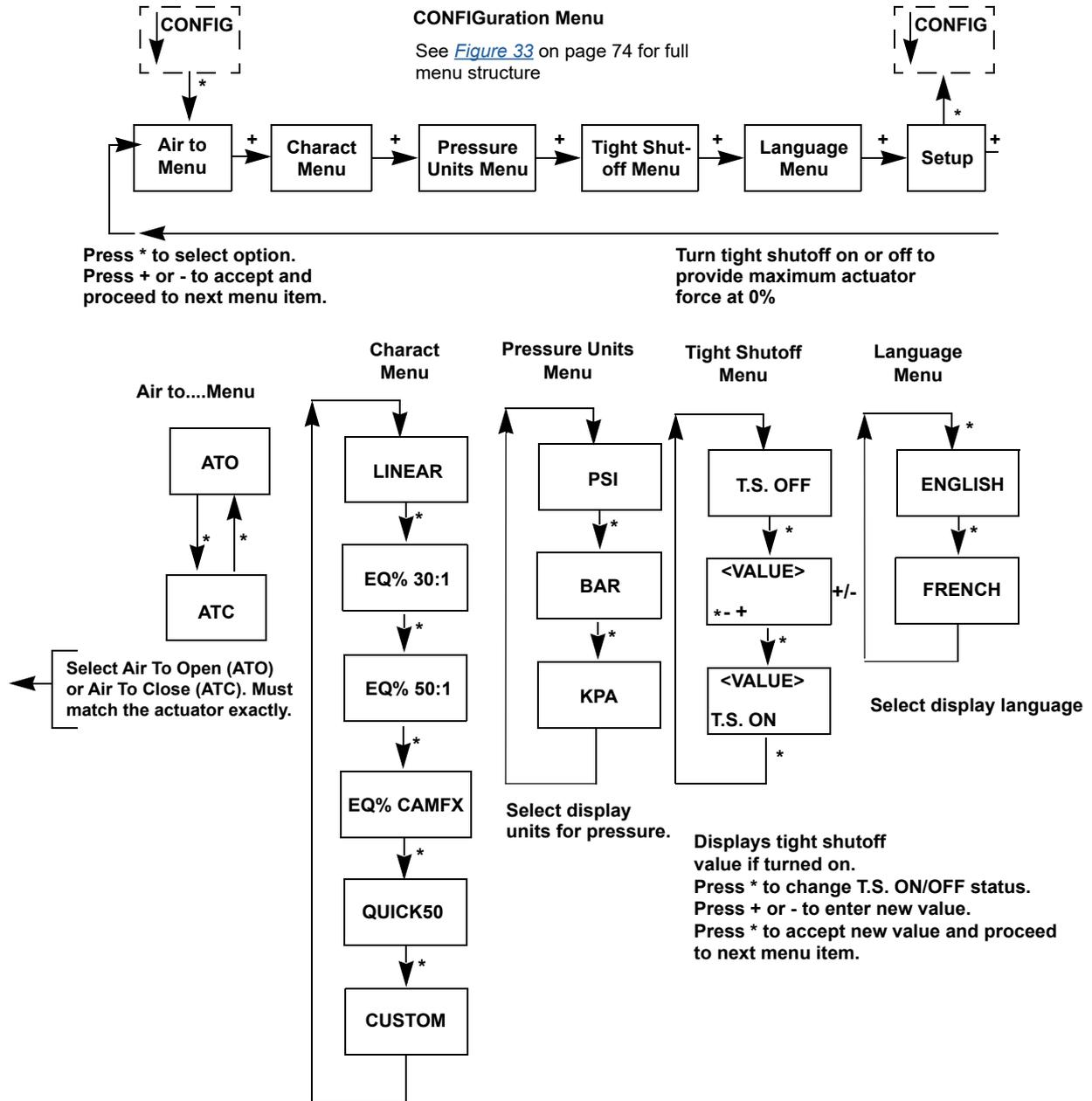
**Figure 39 - Configuration Pushbutton Guide**
