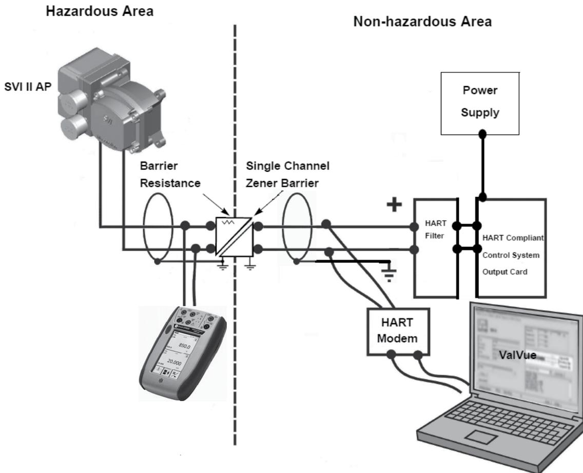
Figure 46 - Intrinsically Safe Installation with Zener Barrier and HART® Filter
