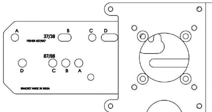
**Figure 30 - Reciprocating Valve Mounting Bracket**
