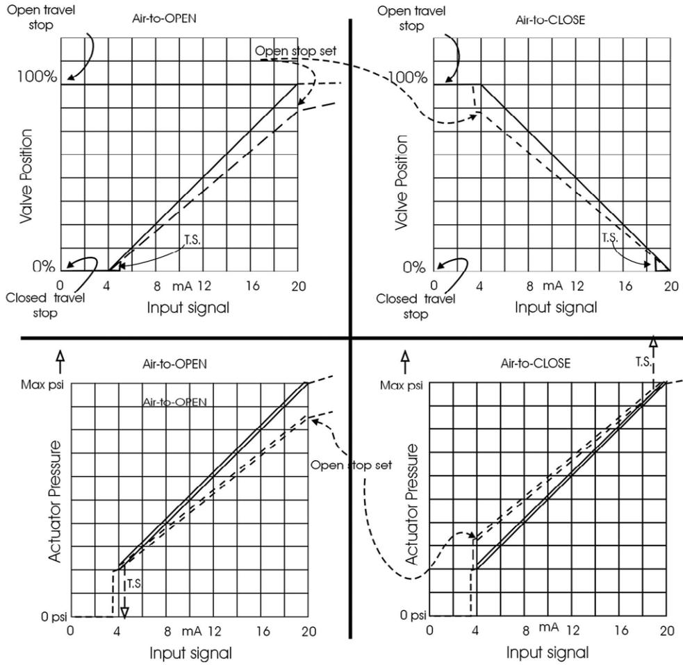
**Figure 63 - ATO and ATC Action with Linear Positioner Characteristics**
