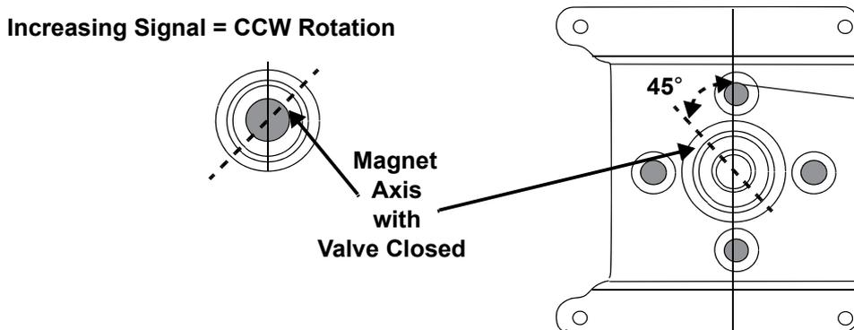
**Figure 28 - Magnet Orientation for 90° Valve Rotation with De-energized Actuator**
