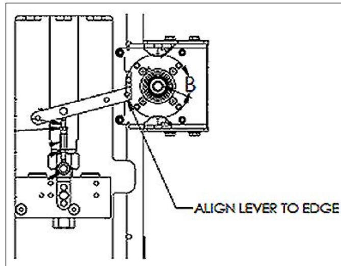
**Figure 22 - Lever Alignment**
