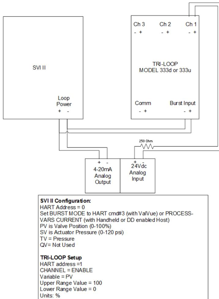
**Figure 71 - Sample Tri-Loop Configuration**
