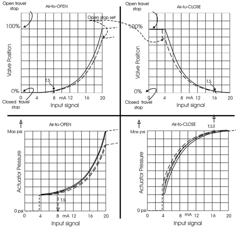
**Figure 64 - ATO and ATC Action in Percentage of Positioner Characteristics**
