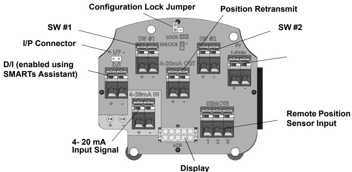
**Figure 31 - Connections to Electronics Module (via Terminal Board)**
