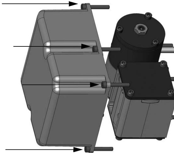
**Figure 59 - Pneumatic Cover Screws: AP (Four Shown)**
