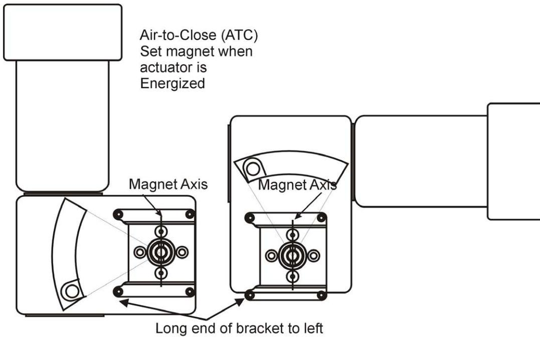
**Figure 12 - Mounting Bracket on Air-to-Close Actuator**
