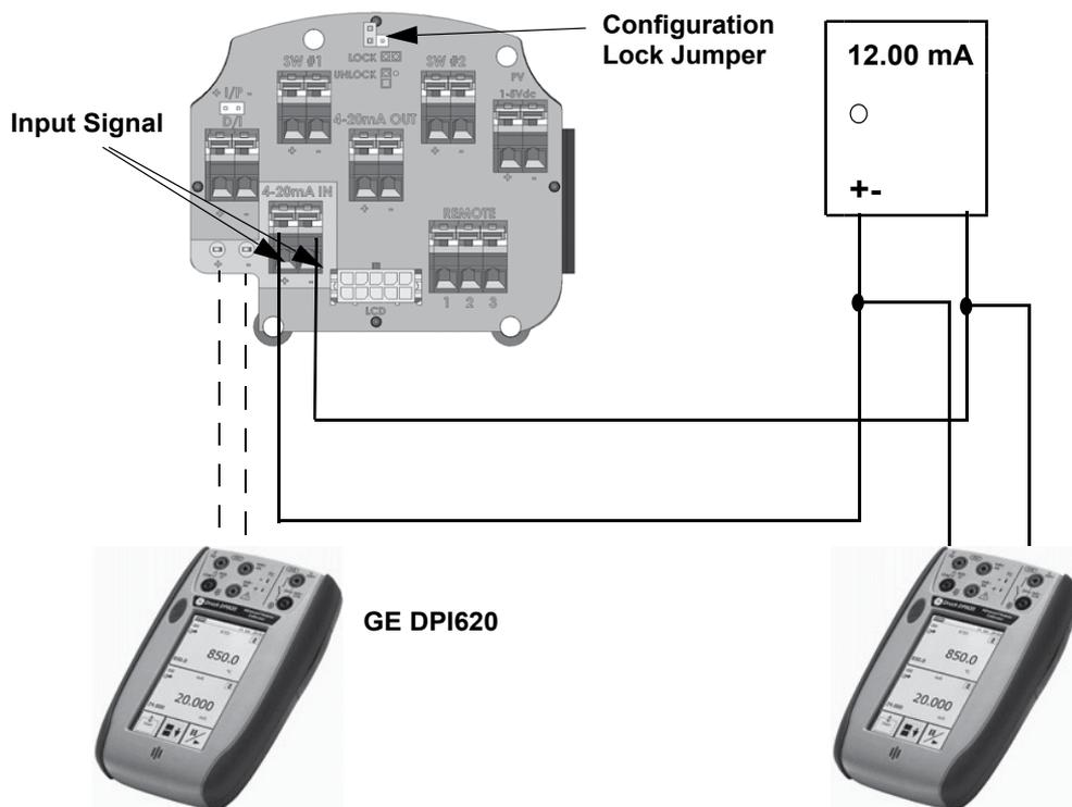
**Figure 41 - SVI II AP HART® Communicator Connections**
