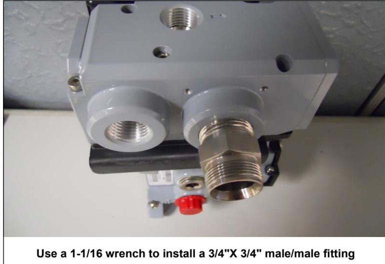
**Figure 68 - Step 1 Install a 3/4" x 3/4" Fitting**
