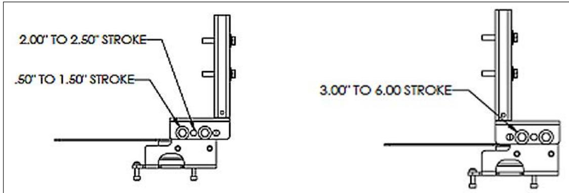
**Figure 20 - Bracket Configuration Strokes .5 - 2.50" and 3-6"**
