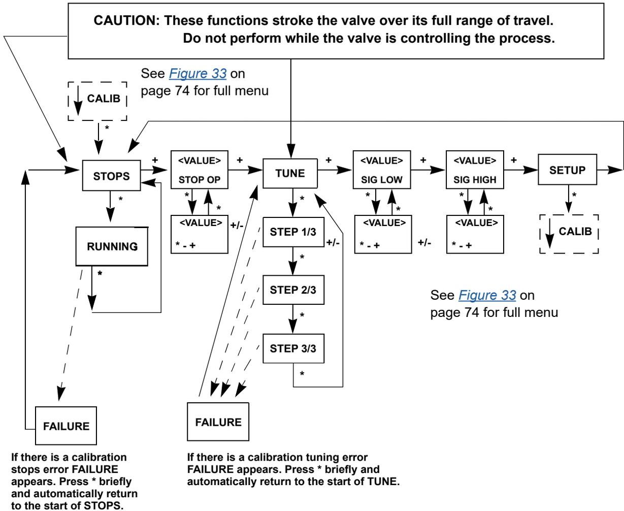
**Figure 40 - Calibration Pushbutton Guide**
