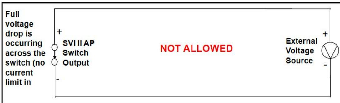
Figure 49 - Switch Installation Drawing without Load: **Configuration Not Allowed**
