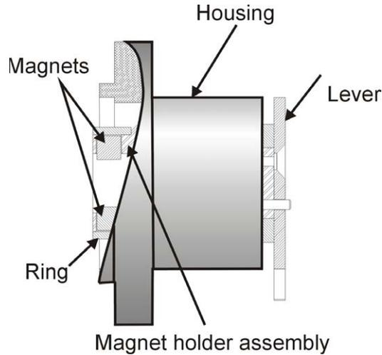
**Figure 14 - Magnet Holder for Reciprocating Valves**
