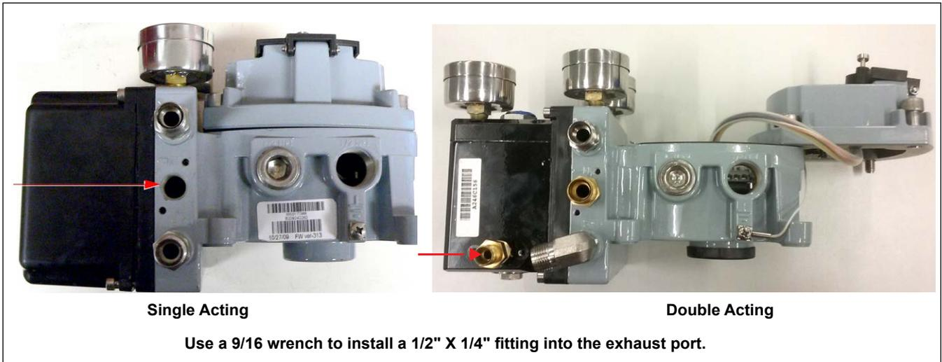
**Figure 66 - Step 2 Install a 1/2" x 1/4" Fitting**
