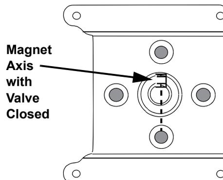
**Figure 27 - Magnet Orientation for Rotary Valves with Valve Closed**
