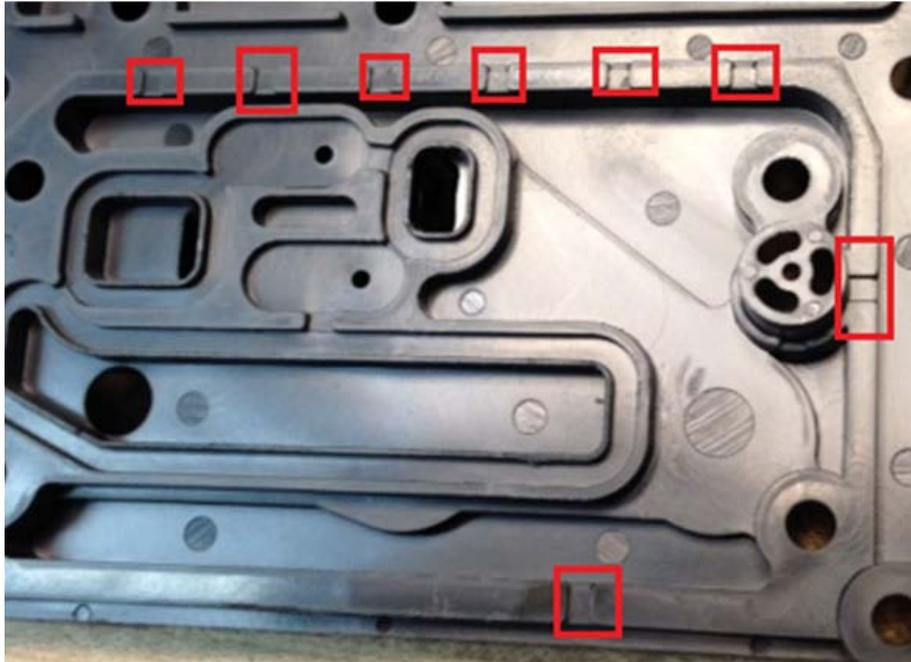
**Figure 55 - Bleed Slots On Air Routing Plate**
