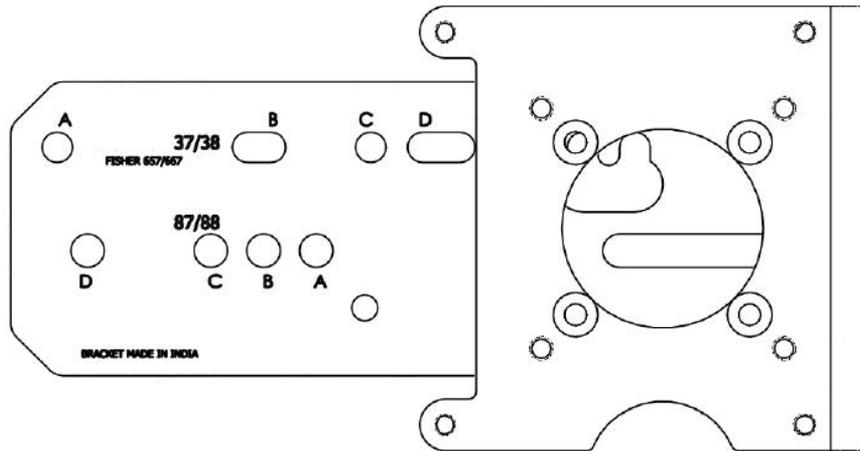
**Figure 15 - Reciprocating Valve Mounting Bracket**
