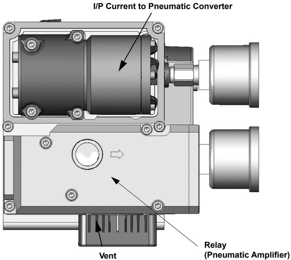
**Figure 53 - SVI II AP High Flow Pneumatic Module with Single Acting Relay**
