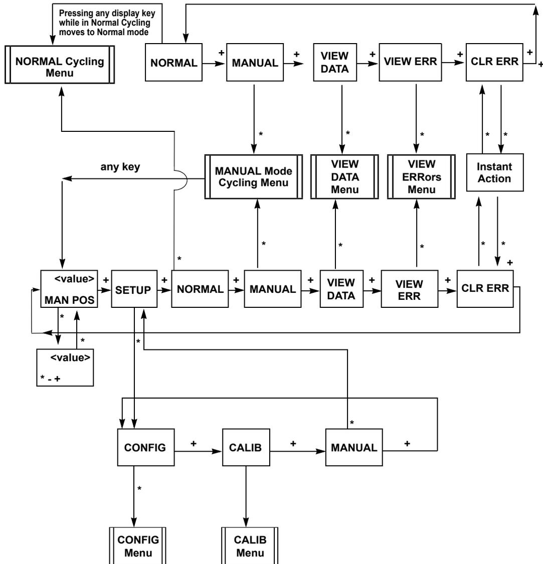
Figure 33 - NORMAL Operation and MANUAL Menu Structures
