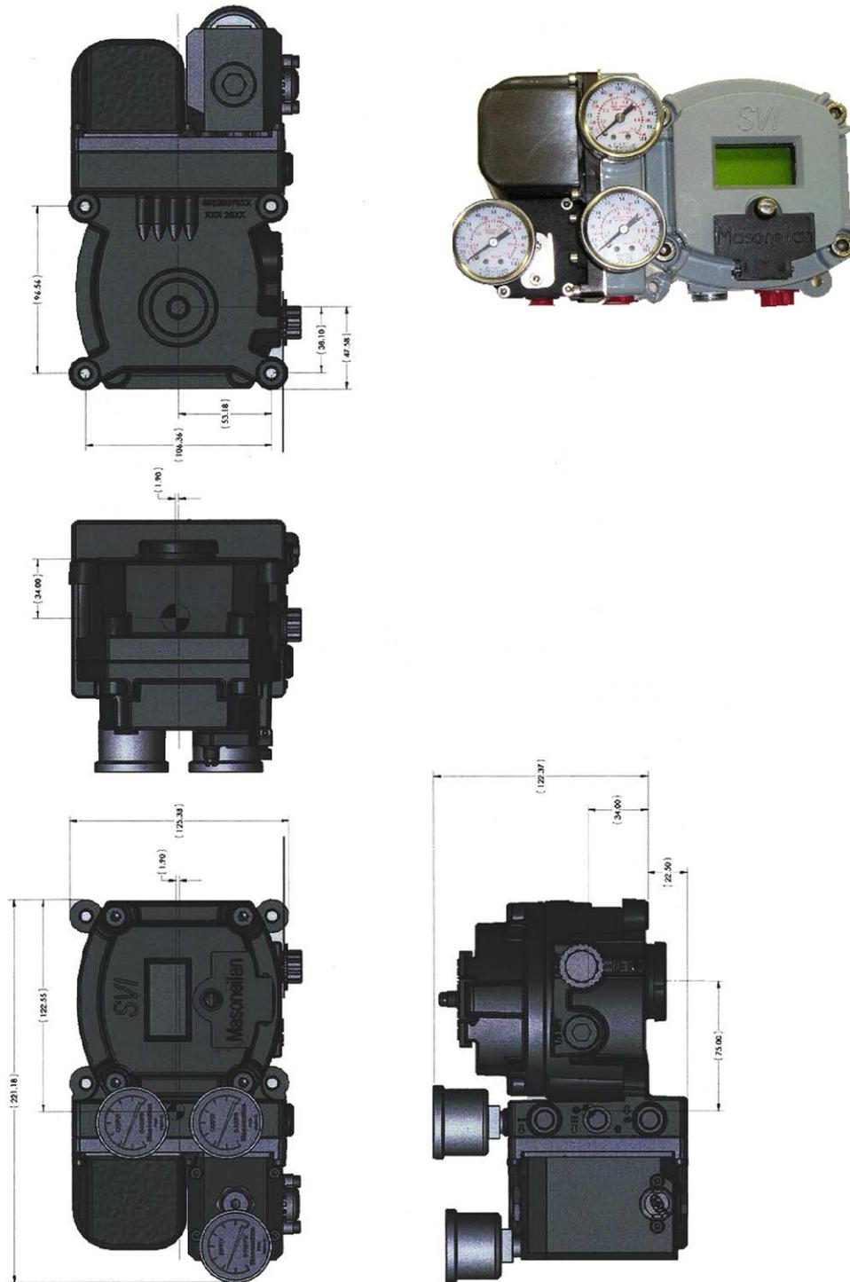
**Figure 8 - SVI II AP Double-Acting Dimensions**
