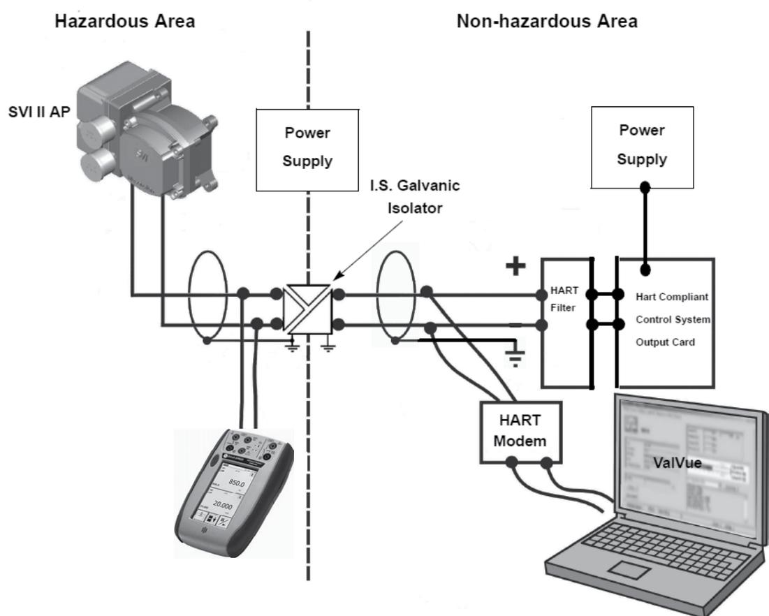
**Figure 47 - Intrinsically Safe Installation with Galvanic Isolator**
