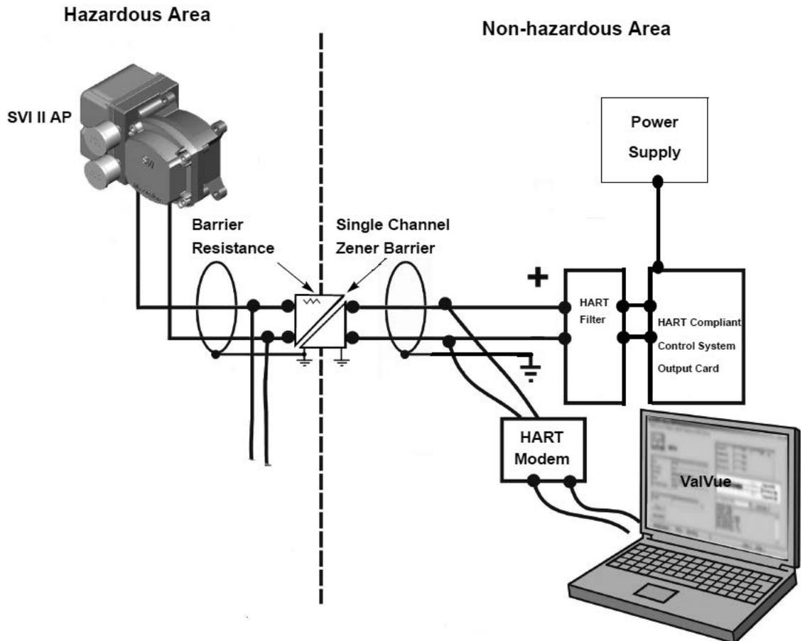
**Figure 43 - Intrinsically Safe Installation**
