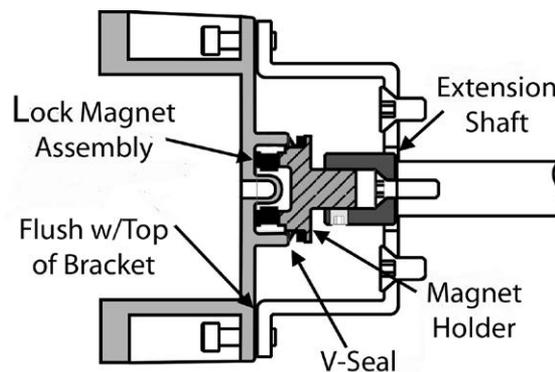
**Figure 10 - Camflex with Mounting Bracket (Side View)**
