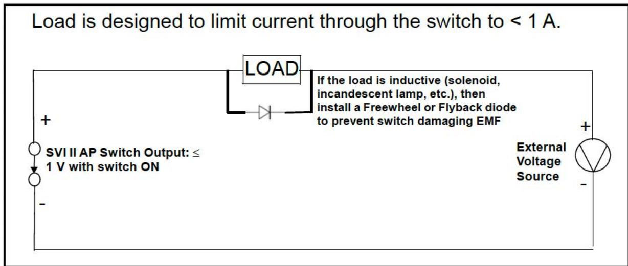
Figure 50 - Switch Installation Drawing: Correct Configuration with Load
