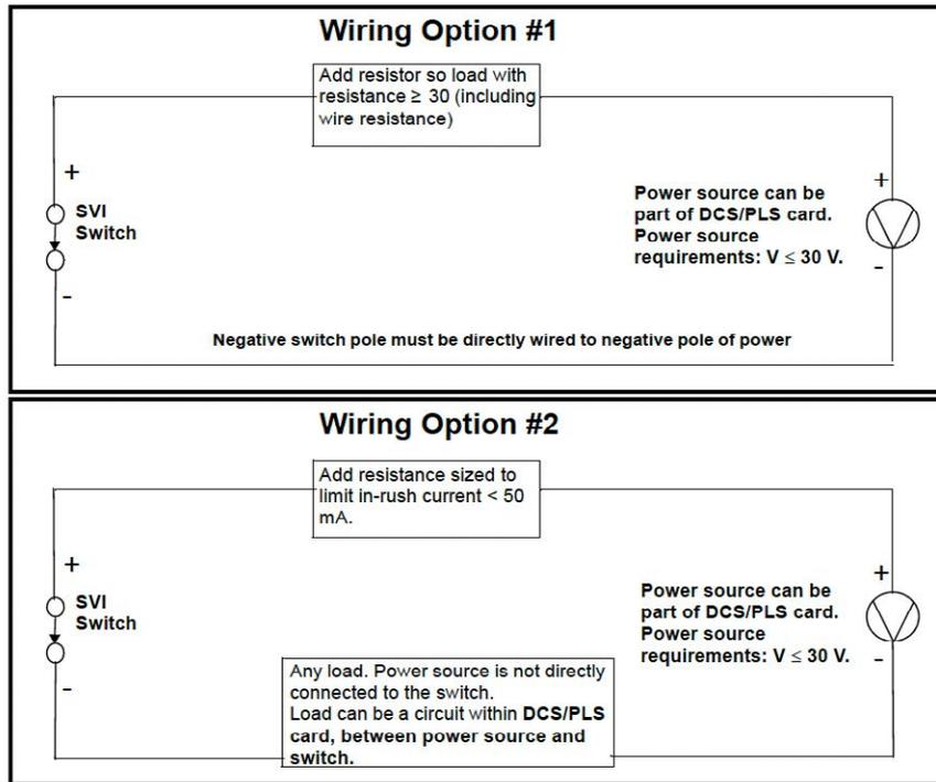
Figure 51 - DCS Switches Wiring Options
