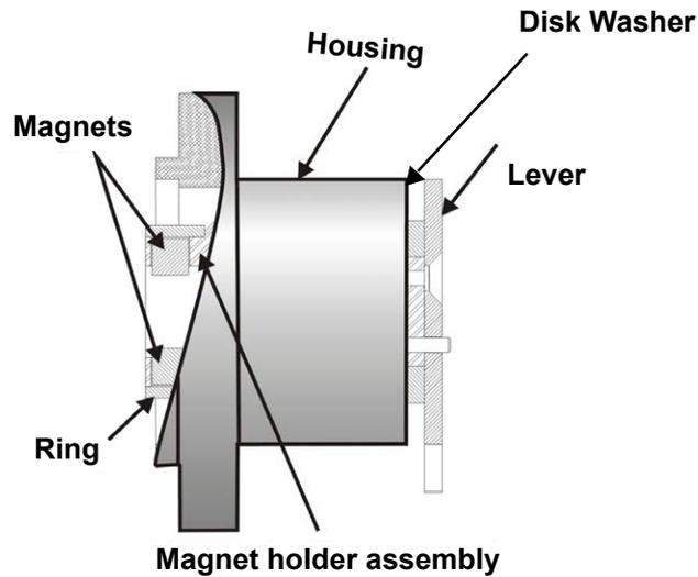
**Figure 29 - Magnet Holder for Reciprocating Valves**
