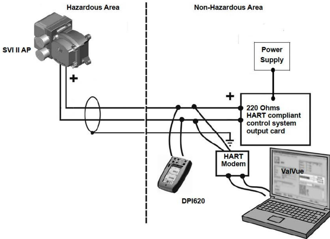
**Figure 42 - General Purpose and Explosion Proof Installation**
