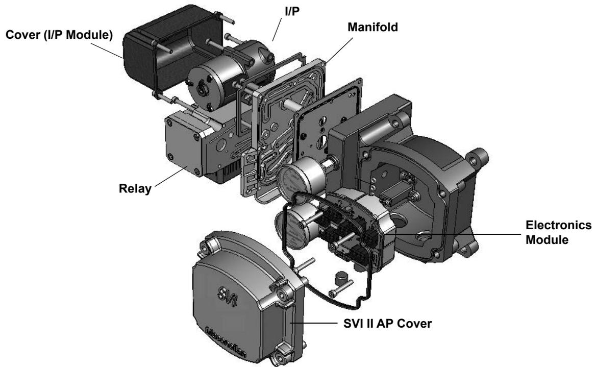
**Figure 6 - SVI II AP High Flow Components**
