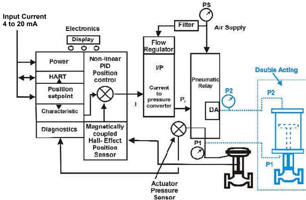
Figure 48 - Block Diagram with I/P Converter and Pressure Sensor
