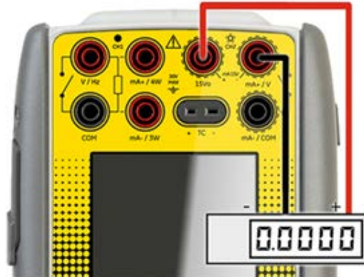
Figure 4-15: Connections for unregulated 15Vo Current Loop Output
