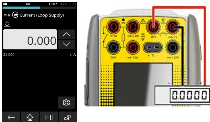
Figure 4-3: Source Current on CH2 with Internal 15V Loop Power, Range 0 to 24mA)
