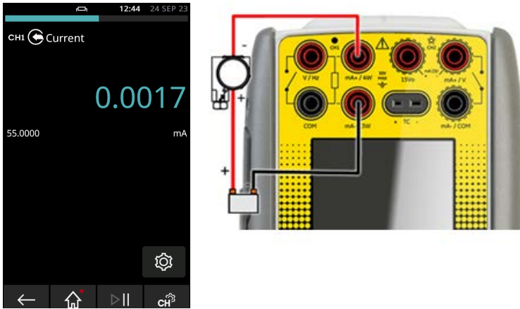
Figure 4-2: Measure Current on CH1 (Range \pm 55\text{mA} )
