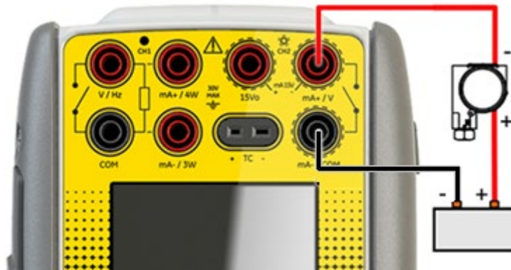
Figure 2-1 Connection with External Loop Supply
