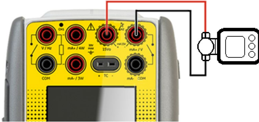
Figure 6-1 Positioner Connection with Internal Loop Supply
