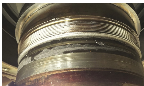
Figure 13. Shaft rub mark in the carbon ring area.
