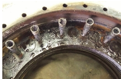
Figure 14. Varnish formation due to oil contamination.
