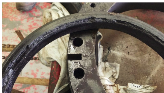
Figure 12. Severe clogging of pollutant on carbon ring faces.
