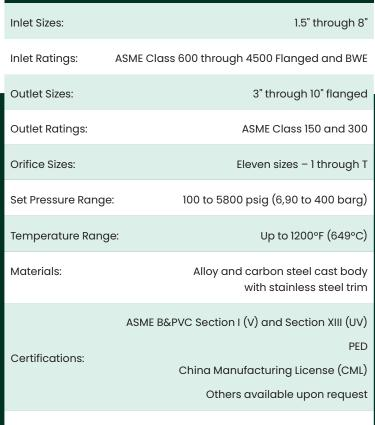
The 1700 Series Maxiflow high-pressure safety valve is a premium product that is installed on a majority of power generating stations worldwide to help protect boilers from overpressure conditions.
