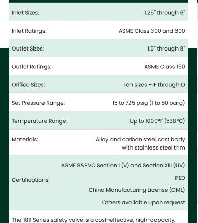
flanged-steel safety valve for steam service.
