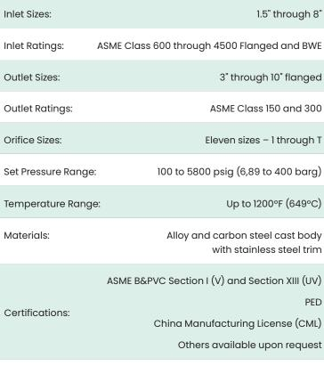
The 1700 Series Maxiflow high-pressure safety valve is a premium product that is installed on a majority of power generating stations worldwide to help protect boilers from overpressure conditions.
