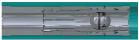
JABS can be deployed in deepwater and high-pressure (15 ksi burst/collapse), high temperature (370°F) environments, gravel-pack operations, horizontal wells, and underbalanced (10 ksi differential across the ball) conditions.
