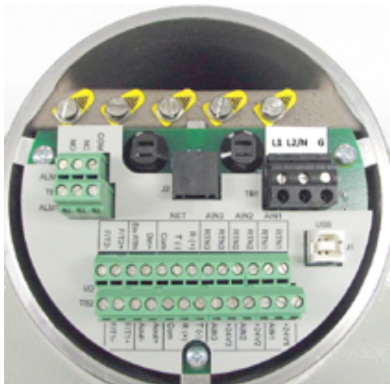
Figure 13: Typical terminal board (three 4-20mA inputs option)
